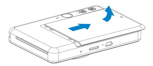
1 Remove the cover by sliding it forward in the direction of the arrow.
